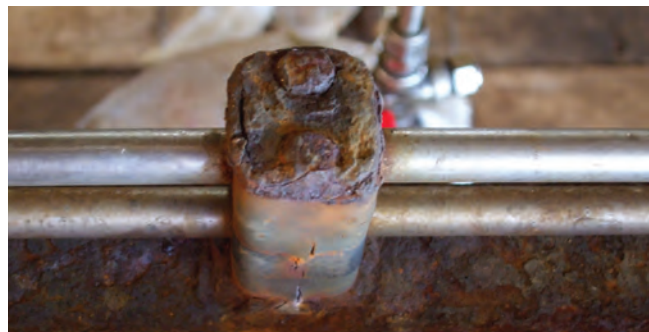
Crevice corrosion between the tube/tube trap interface.
