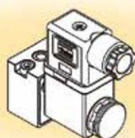
Valve is fitted with a 30mm solenoid having DIN 43650 Industrial form A. Operator body in thick anodised aluminium, stainless steel screws and armature allows compatibility with Railway applications.
