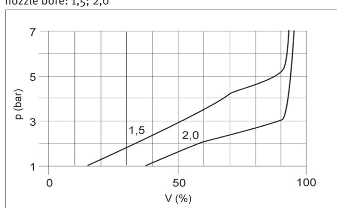
p= propulsion water pressure (bar)
