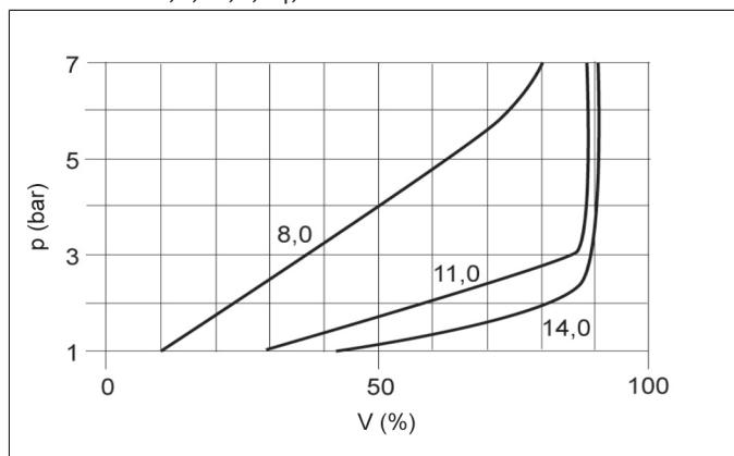
*p= propulsion water pressure (bar)*
