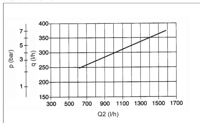
p = propulsion water pressure (bar)
