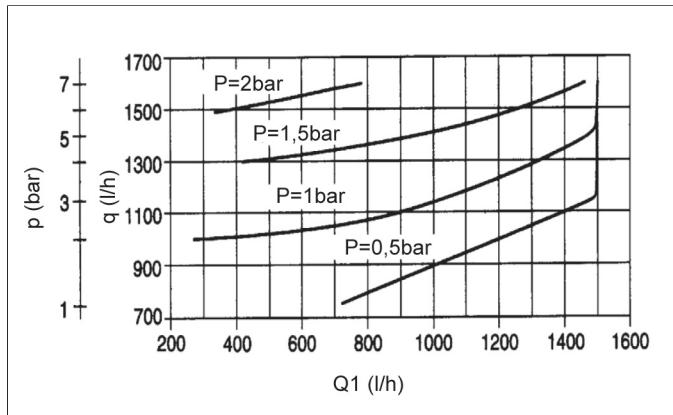
p = propulsion water pressure (bar)
